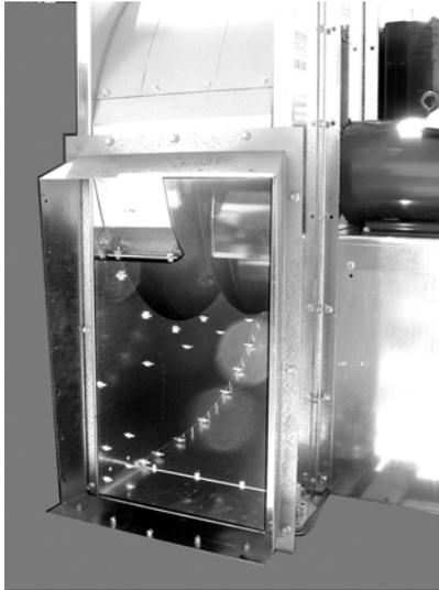
Align the Transition at the Frame end and bolt to the Adapter Plate. Place hardware in the **inner** holes first. Align **outer** hole patterns in the Plate with holes in the Fan end of the Transition.
